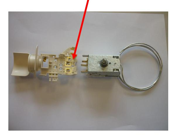
Bend the rear side of the lamp holder with 90 degrees, so that it fits the plug connections of the thermostat!
