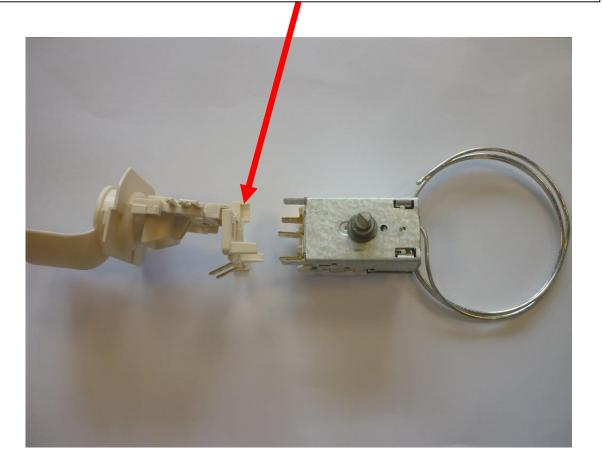
Bend the rear part of the lamp holder with 90 degrees, so that it fits the plug connections of the thermostat!
